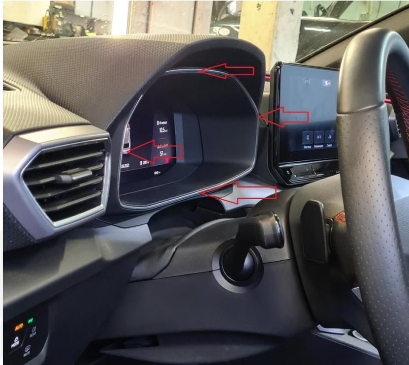
**Step 3:** Open top cover from the steering colom bij putting a flat screwdriver of something else on the following location and **on both sides.**
