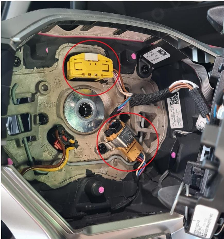
**Step 8:** Remove connector from steering wheel heating iff you have this steering wheel.
