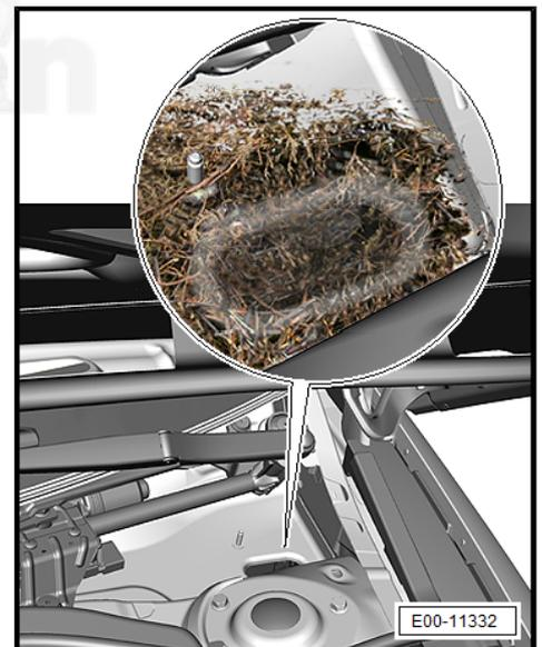
An accident where the vehicle body has been exceptionally deformed may also have damaged the sealant between the sheet metal thus allowing water to enter.
