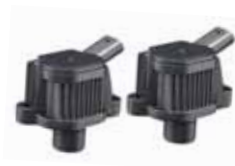
Cylinders 2 and 3 intake cam actuators, N583, N591 .
