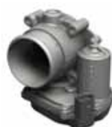
Butterfly throttle valve control unit, J338 Butterfly throttle sensors 1 and 2 (accelerator electronic control) G187, G188
