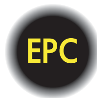
Electronic accelerator control warning light, K132
